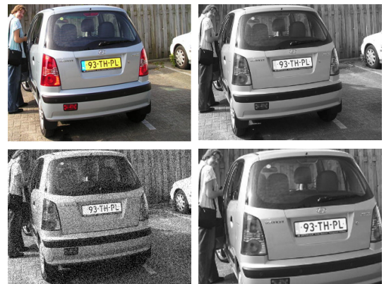
Fig. 3: A typical image with a license plate to be recognized. a) original, b) grey-scaled, c) added 10% noise, d) zoomed in by 40%
